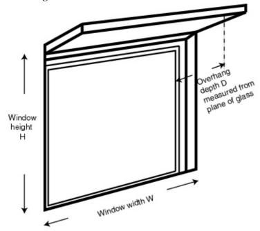
Where the overhang is at least twice as wide as the window (e.g. balconies on blocks of flats) use Table P4. In other cases use Table P5. Interpolation may be used between rows of these tables. Use the average overhang depth if it varies. Usually the same value of  $Z_{\text{overhangs}}$  can be applied to all the windows on a given façade on the basis of an average depth-to-height ratio. This can be applied only to windows whose orientation is known.
